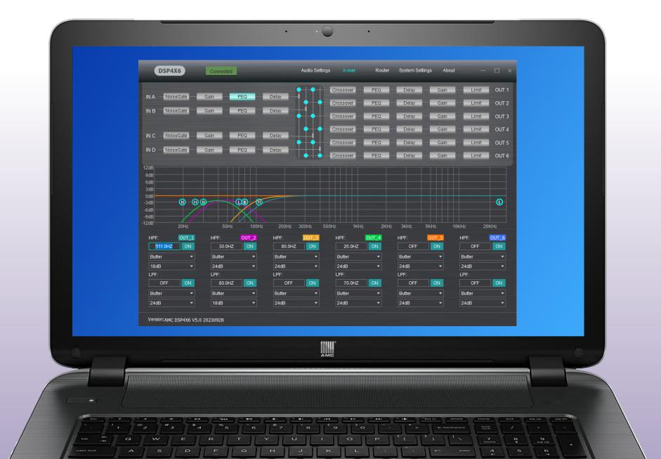
3. Dynamic processing: 10 points parametric EQ, crossover, input gate, compressor, limiter and signal delay.
