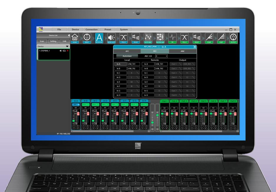
4. Each channel features dynamic processing: parametric EQ, crossover, input gate, compressor, limiter and delay.
