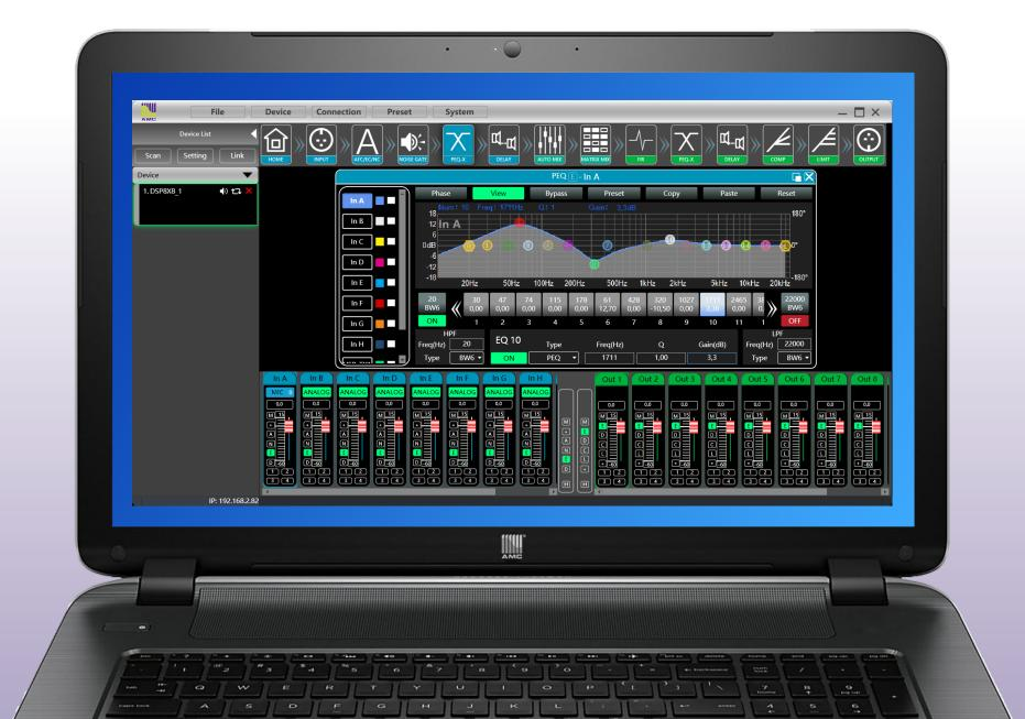
5. FIR filter designer. Advanced feature for signal processing without phase distortion.
