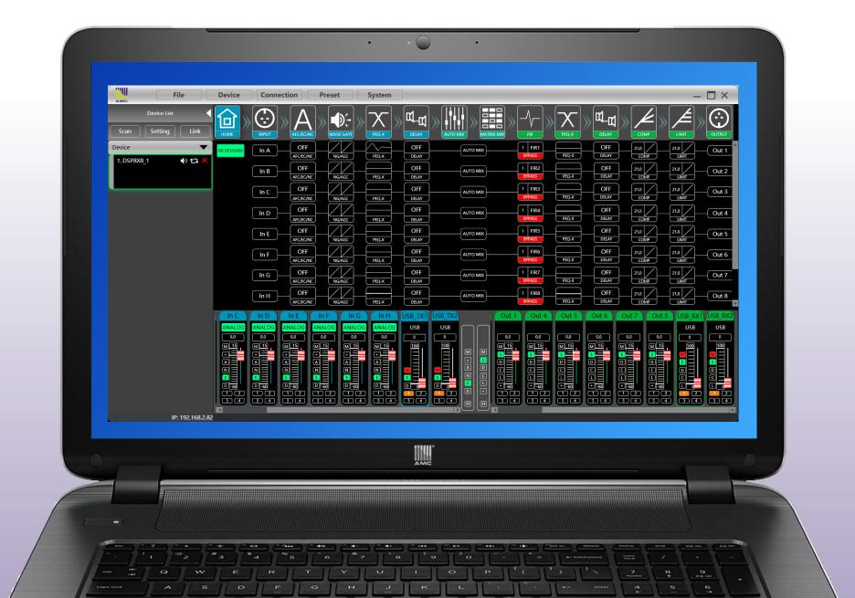
2. DSP8X8 can use MIC/Line level balanced inputs, providing phantom power, gain control and phase invert setting. For system testing purposes, a test signal (noise or wave) can be generated internally and assigned to any input channel.
