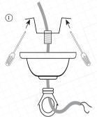
Route the cable through all parts of mounting bracket.
