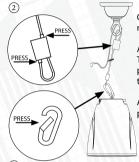
Connect provided steel rope to the mounting bracket and the speaker.
