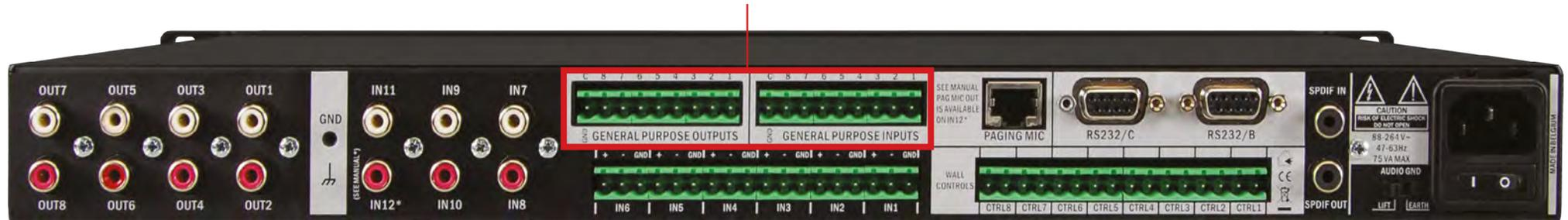
The **AC12.8SET** offers additional features like message player, general purpose inputs & outputs, output delay and zone combining.
