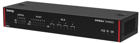
The Tango is equipped with three bi-directional RS-232 interfaces for sending commands to AV devices with feedback functionality. It is additionally equipped with 2 uni-directional RS-232 interfaces for sending commands to AV devices using serial or infrared communication. 8 GPIO are available for control of relays, switches, and sensors. Impera Tango is an adaptable AV control system for medium and large conference rooms.
